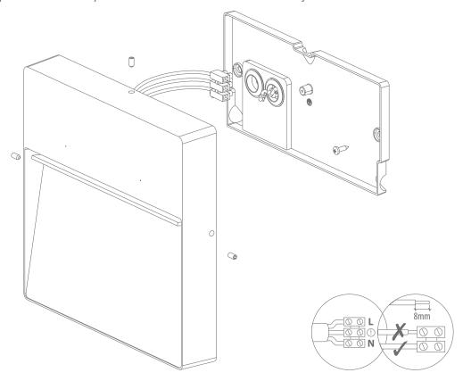
**Note:** -The lamp must be installed by professional electrician
