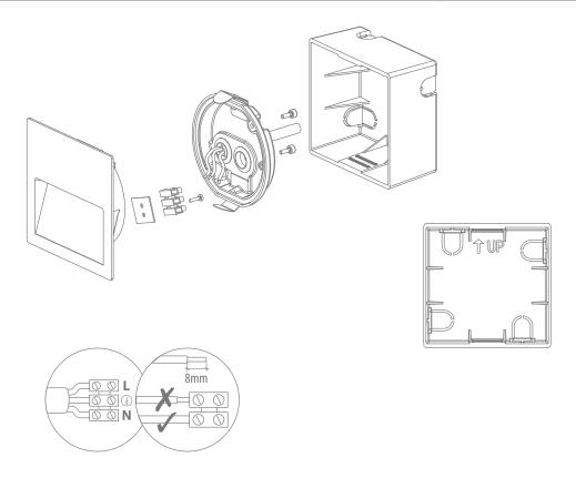
Cutout without recessed box: (L) 100mm x (W) 100mm Cutout with recessed box: (L) 110mm x (W) 110mm
