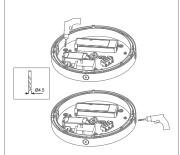
4. Connect the wires to the block through the reliefs
