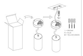
2. Determine mounting location and knock the plastic anchor into ceiling, fix the bracket and screw into ceiling.
