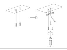
4. Properly align the mounting holes between back plate and mounting bracket, then lock them together with screw,
