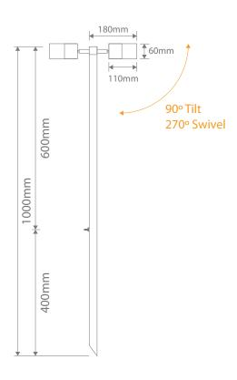
**Note:** -The lamp must be installed by professional electrician
