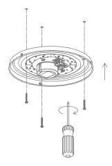
3. Connect the wire to terminal at base plate, and ensure correct connection is made. Replace terminal block cover.
