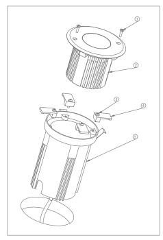
1. Drill a hole with the diameter of Ø115 in the ground.
