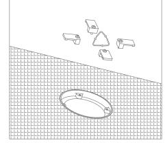
4. Insert the luminaire (2) into the housing (5). Fasten luminaire (2) to housing (5), using the screws (1) provided.
