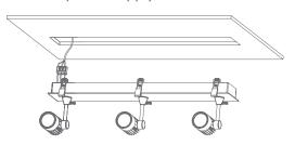
3. Hold the spring clips upwards and insert spotlight into position
