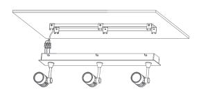
4. Hang the spotlight of bracket and tighten screws
