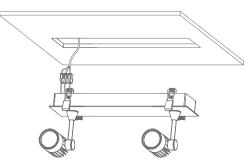
3. Hold the spring clips upwards and insert spotlight into position
