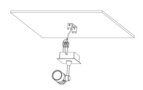
4. Hang the spotlight of bracket and tighten screws
