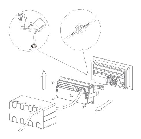
Must use round rubberised flex cable through the cable gland.
