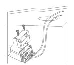
Connect the downlight with driver, hold back the spring clip then push the downlight into the hole.
